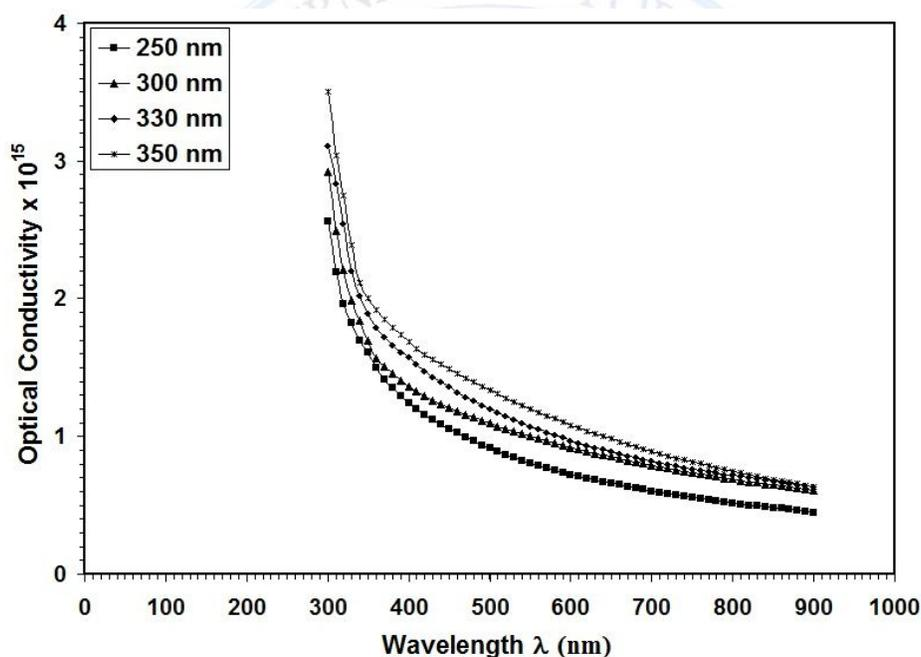
Fig. (5) Optical conductivity versus wavelength for SnO<sub>2</sub> films.
