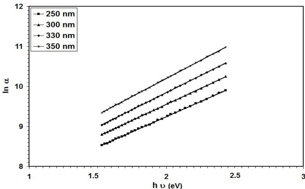
Fig. (2)  $\ln \alpha$  versus photon energy for SnO<sub>2</sub> films.
