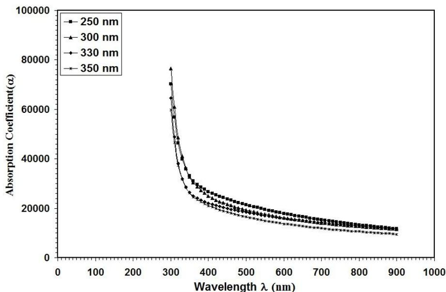
Fig. (1) Absorption coefficient versus wavelength for SnO<sub>2</sub> thin films.
