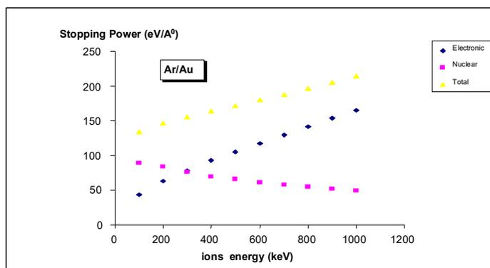
Fig(1):stopping Power versus Ar ions energy
