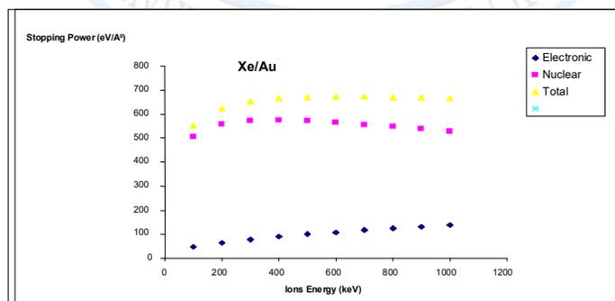
Fig(3):stopping Power versus Xe ions energy
