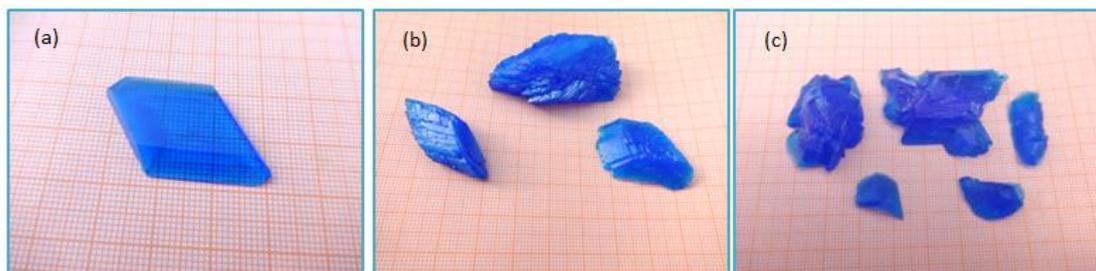
**Figure 2:** Photographs of single crystals (a) Distilled water. (b) Diluted  $H_2SO_4$  acid.
