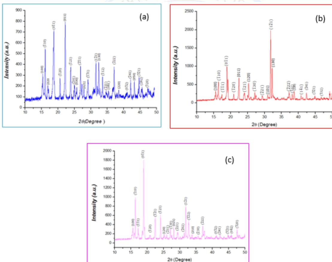
**Figure 3:** PXRD patterns of grown crystal by (a) distilled water, (b)  $H_2SO_4$  acid, (c) magnetic water as a solvent
