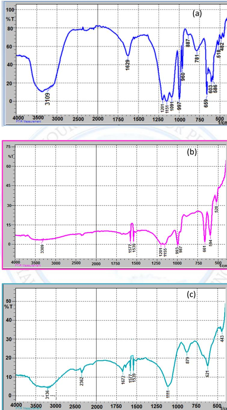
Figure 4: FTIR transmission spectra of crystals grown using (a): Distilled water. (b): H<sub>2</sub>SO<sub>4</sub> acid. (c): Magnetic water
