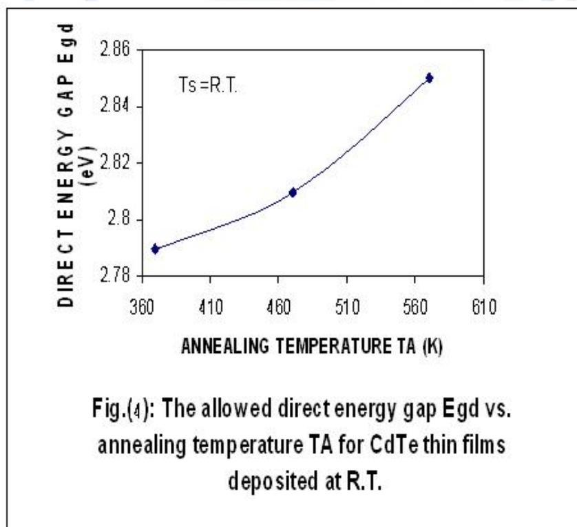
Fig.(4): The allowed direct energy gap  $E_{gd}$  vs. annealing temperature  $T_A$  for CdTe thin films deposited at R.T.
