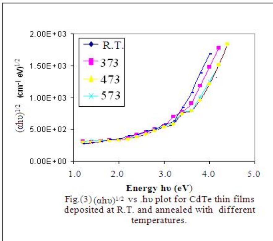
Fig.(3)  $(\alpha h\nu)^{1/2}$  vs.  $h\nu$  plot for CdTe thin films deposited at R.T. and annealed with different temperatures.
