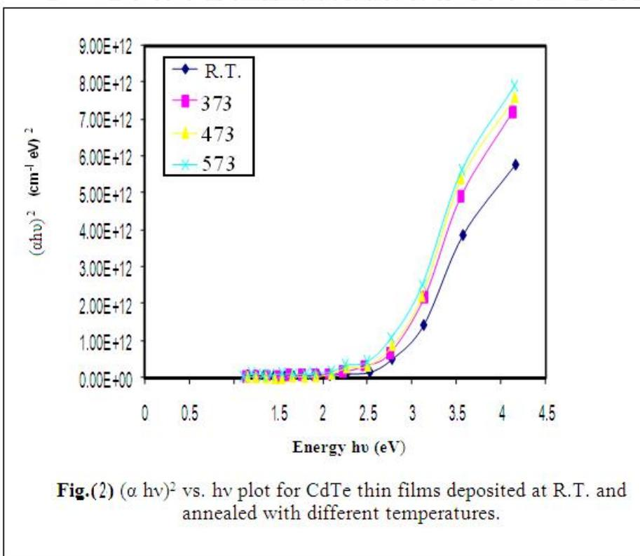
Annealing effect on the optical energy gap of (CdTe) thin films
