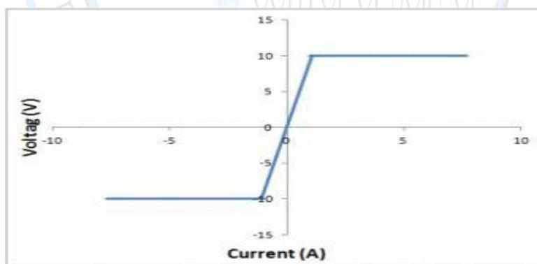
**Figuer(6):The I-V characterization of nano Ag thin film( 60,65)nm on glass substrat.**
