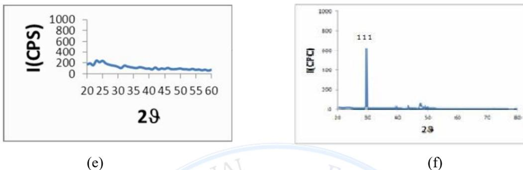
Figure (2): XRD pattern of nano Ag thin film ( 46)nm on silicon substrate (e) before (f)after sintering.
