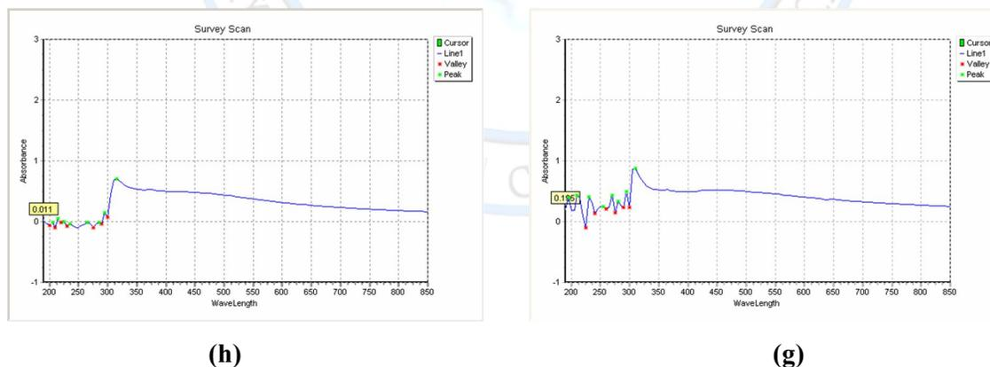
Figure(3): The UV-vis. spectrum of nano Ag thin film (g)( 60 )nm, (h)( 65)nm on glass substrate.
