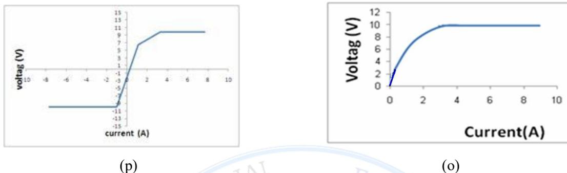
**Figuer(7): The I-V characterization of nano Ag thinfilm( o-41,p-46)nm on Si substrat.**
