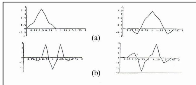
**Figure (1): GHM pair of, (a) Scaling Functions, (b) Multiwavelets**
